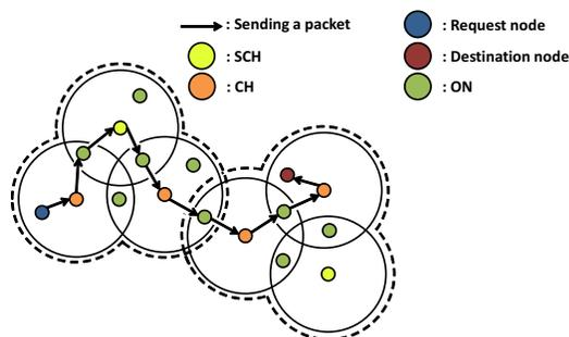
Figure 6. A communication path in the second approach.
